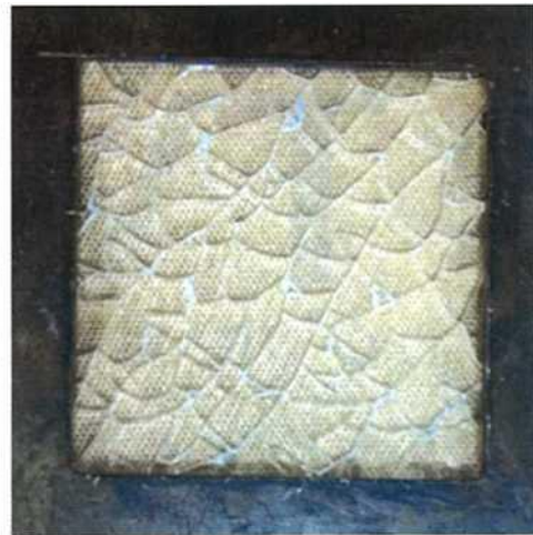
图 40: 37#样品碎片状态 Fig. 40: Fragmentation of the sample 37#
